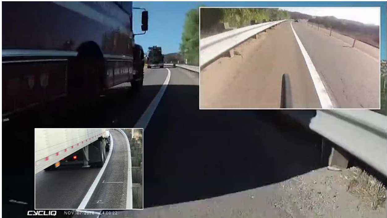
Figure 8. Uphill northbound, 1 lane, rumble strips, center delineators, narrow shoulders, EXTREMELY DANGEROUS.
