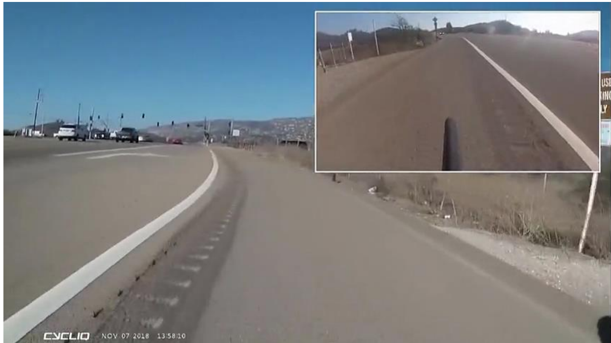
Figure 7. At Poway Rd northbound, through cyclists trapped by rumble strips right of right turn lane to trailhead parking
